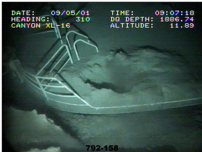
Figure 5-38. Sediment on Bow After the Stern Lift Viewed from Above Port Bow.
