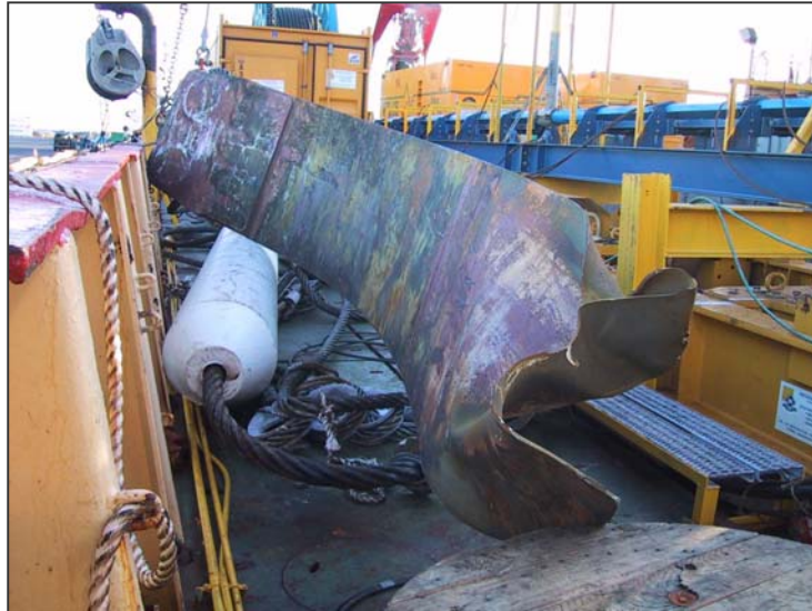
Figure 5-35. Broken Lifting Plate After Stern Lift.
