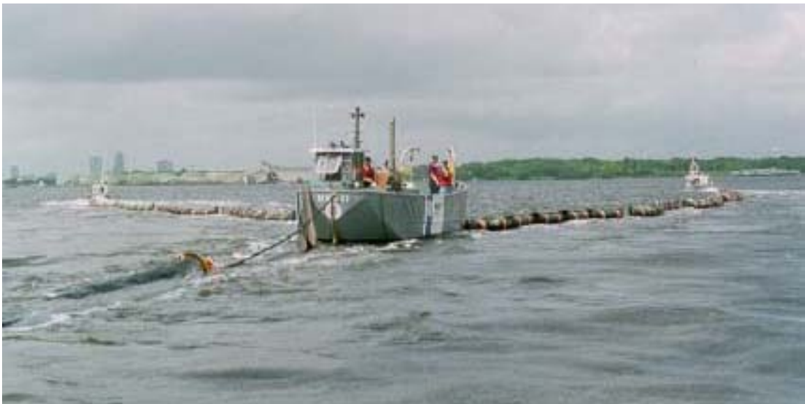
Navy SUPSALV Offshore Skimmer System – Note forward end of oil storage bladder in left foreground, skimmer vessel in center with oil containment “V-booms” forward of the skimmer all towed by a pair of towing vessels
