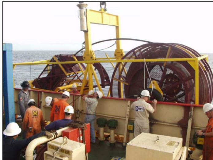
Figure 5-33. Coiled-Tubing Drilling System Being Deployed.
