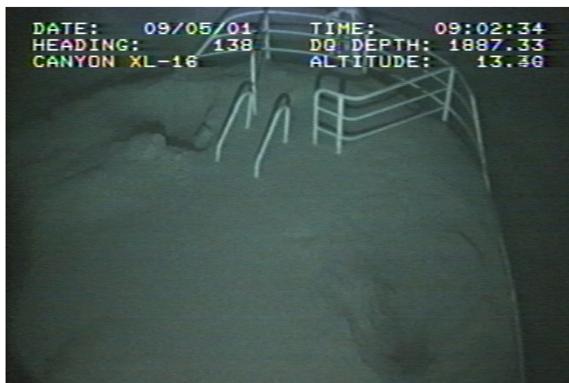
Figure 5-39. Sediment on Bow Viewed from Above Starboard Bridge Wing.
