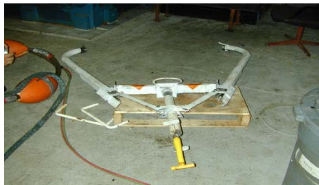
Figure 5-22. Shaped Explosive Charge Tool in Expanded Position to Allow for Going Around the Mast.
